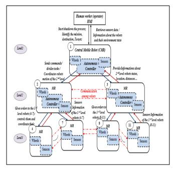
Fig. 7. The modified hierarchical architecture of our system.
