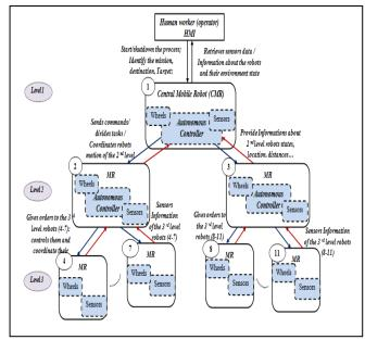
Fig. 6. The hierarchical architecture of our system (the blue color refers to orders and the red color refers to feedback).
