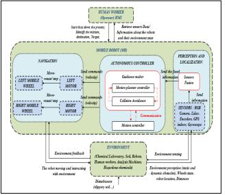
Fig. 4. The detailed control architecture for one robot with two differential wheels.
