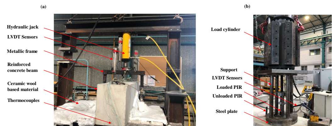
Figure 2. Testing apparatus in the heating phase (a) and the cooling phase (b).
