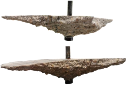
Figure 5: Typical failure cone
