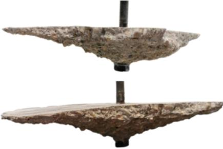
Figure 5: Typical failure cone
