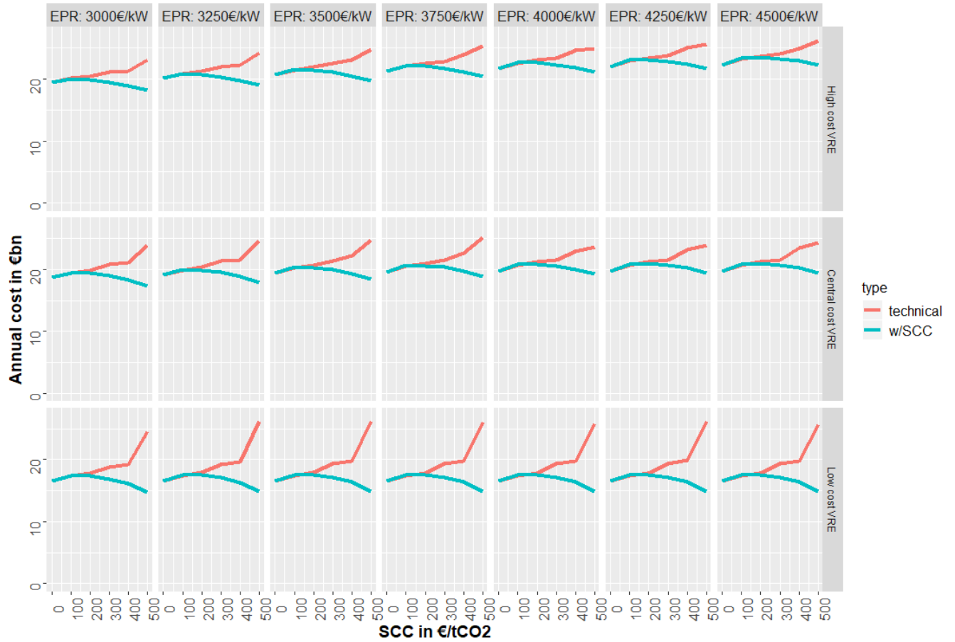
Figure 11. Annualized technical cost and cost with social cost of carbon (including SCC) for different VRE and nuclear power cost and SCC scenarios for 2050
