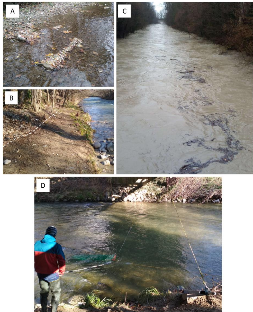
Figure 2. Pictures of the Lower Lysse River at the university bridge. (A): riverbed at low flow with litter accumulations upstream of boulders (13 November 2018, Q : 1 \text{ m}^3 \text{ s}^{-1} , water depth: 20 cm, width: 14 m); (B): river bank on 19 March 2019, after a high flow event. The white dotted line indicates the highest level reached by the stream. (C): Brown turbid water during a rising limb at very high flow ( Q : 170 \text{ m}^3 \text{ s}^{-1} , water depth: 3.4 m, width: 20 m) with floating logs and branches in the middle of the river; (D): sample collection using the hanging net technique during a falling limb ( Q : 9.4 \text{ m}^3 \text{ s}^{-1} , water depth: 0.8 m): note the water transparency.
