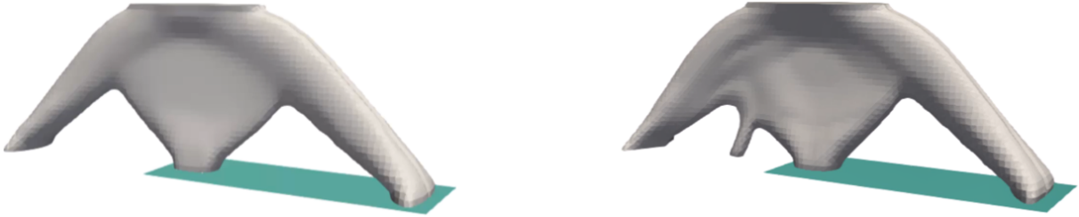
Figure 17: Initial geometry (left) and optimized (right) for minimizing (25) after the partial cut.
