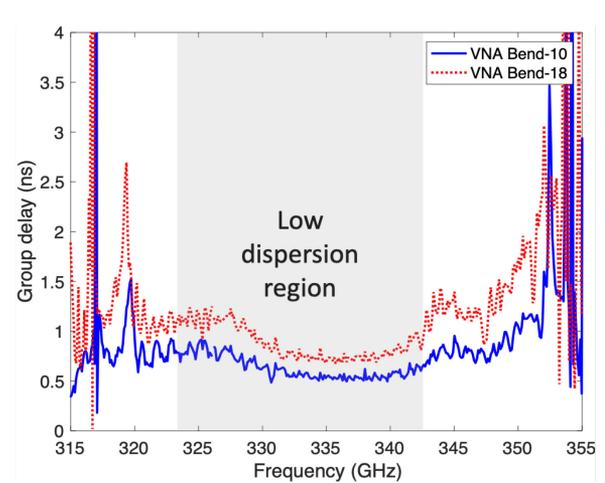
Fig. 13. Group delay from VNA measurement for 10-bend and 18-bend. The gray low-dispersion region is as defined from the simulation result in Fig. 8.
