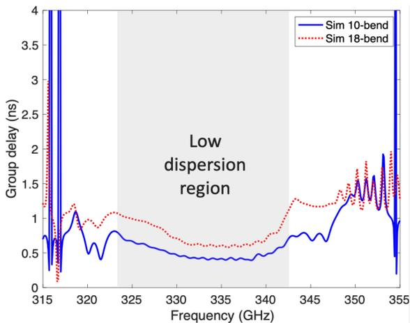
Fig. 8. Group delay from EM simulation for 10-bend and 18-bend. The low-dispersion region is in agreement with the low-loss region in Fig. 6.
