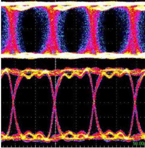
Fig. 15. Eye-diagrams at (top) pre-amplifier output and (bottom) limiting-amplifier output for 10 Gbit/s ASK modulation.
