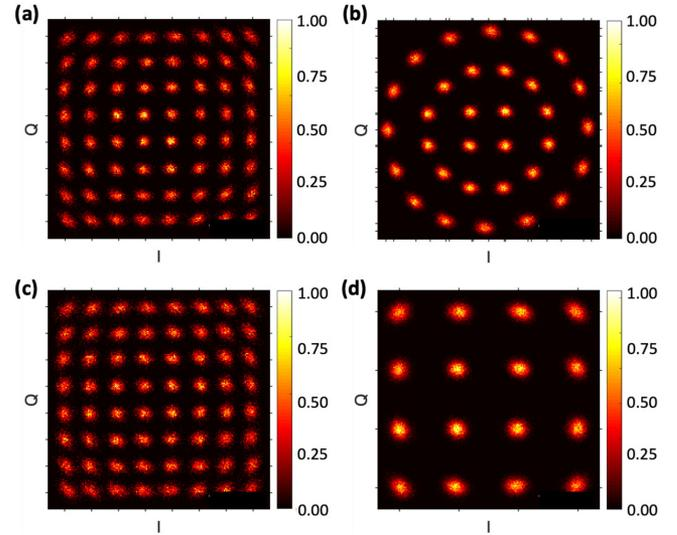
Fig. 17. I-Q intensity constellation diagram for recovered symbols: for 10-bend (a) 60 Gbit/s using 64-QAM, (b) 60 Gbit/s using 32-APSK, (c) 75 Gbit/s using 64-QAM, and (d) 50 Gbit/s using 16-QAM. The intensity scale on the right indicates the 3-dimensional distribution of I-Q points over multiple frames.
