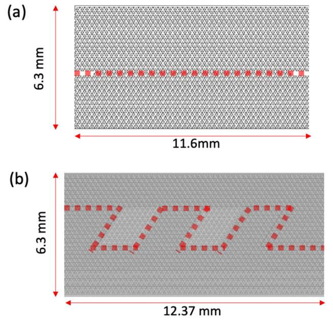
Fig. 3. Schematic of VPC waveguide for (a) 10 mm straight and (b) 10-bends. The dashed red-line indicates the waveguide light path.
