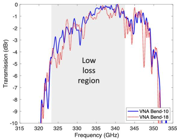
Fig. 11. Transmission from VNA measurement for 10-bend and 18-bend. The gray low-loss region is as defined in Fig. 6.
