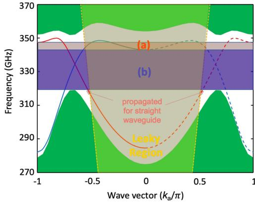
Fig. 2. Dispersion diagram for the first Brillouin zone showing (a) bandgap with linear dispersion for the Large zigzag used in straight sections and (b) bandgap for the Small zigzag additionally employed in the diagonal bend sections. The red and blue lines represent the edge dispersion of Large and Small zigzag waveguides respectively. The light-line in air is indicated by the yellow dashed line.
