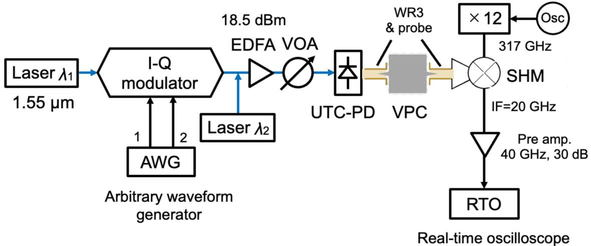
Fig. 14. Block diagram of the I-Q communications experiment. The VPC waveguide tapers interface between the uni-traveling carrier-photodiode (UTC-PD) Tx and sub-harmonic mixer (SHM) receiver using probe extenders.
