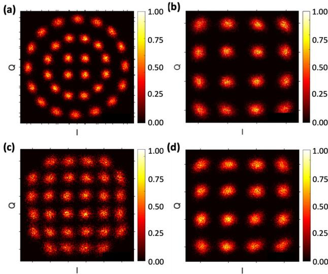
Fig. 16. I-Q intensity constellation diagram for recovered symbols: 10 mm straight at (a) 100 Gbit/s using 32-APSK, (b) 100 Gbit/s using 16-QAM, (c) 125 Gbit/s using 32-QAM and (d) 108 Gbit/s using 16-QAM. The intensity scale on the right indicates the 3-dimensional distribution of I-Q points over multiple frames.
