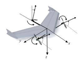
Fig. 26. Tri-copter with laterally tiltable tail propeller [118].
