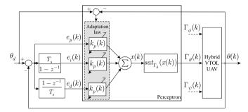
**Fig. 19.** The pitch angle control architecture used in [113]. The pitch torque  $\Gamma_{\theta}(k)$  applied to the aircraft is computed from the pitch angle error  $e_{\theta}(k) = \theta_d(k) - \theta(k)$  and passed through a PID controller whose gains are adapted on line, as being the weights of one-neuron neural network.
