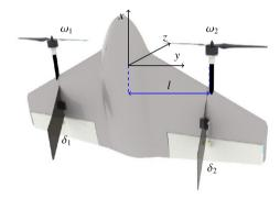
Fig. 24. Tailsitter simultaneous rotor and elevon allocation example [57].
