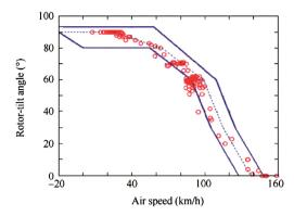
**Fig. 10.** Tiltrotor UAV flight envelope. Rotor-tilt angle as a function of airspeed [58, 144,147].
