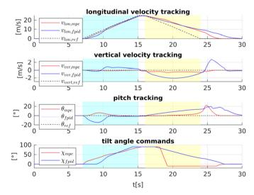
**Fig. 22.** Simulation results comparing NMPC and FPID performance during transition phases with acceleration and deceleration phase highlighted in cyan and yellow, respectively.
