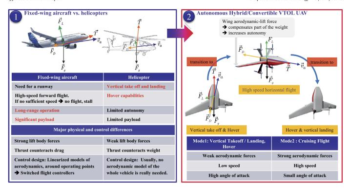
Fig. 1. Fixed-wing aircraft vs. helicopter vs. a possible hybrid-VTOL aircraft: main properties. The respective advantages of fixed-wing aircraft and helicopters are highlighted in red. (For interpretation of the colors in the figure(s), the reader is referred to the web version of this article.)
