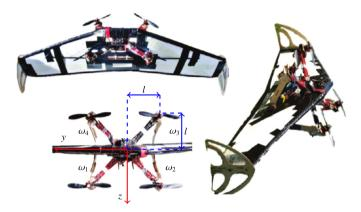
Fig. 23. Tailsitter with four rotors, no elevon [78].
