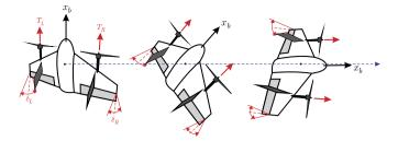
Fig. 9. Transition maneuver of a tailsitter aircraft at constant altitude.
