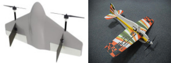
(a) Left: Flying-wing design [57]. Right: Wing-fuselage design [35].
