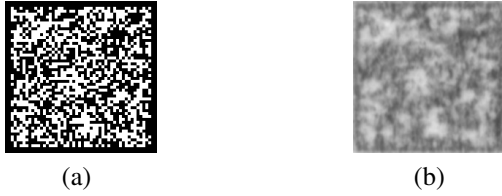
Fig. 1. Example of CDP a) an original random binary image before printing ( I ) and b) its degraded by P&S version ( \tilde{I} ).
