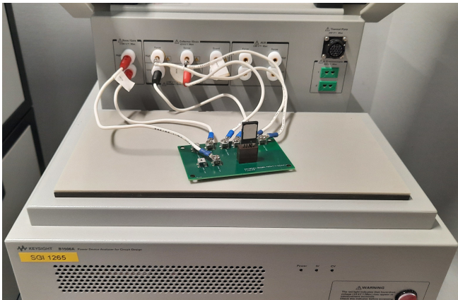
Fig. 2: Connection on the B1506A of a custom-built board for TO-247-4 packages
