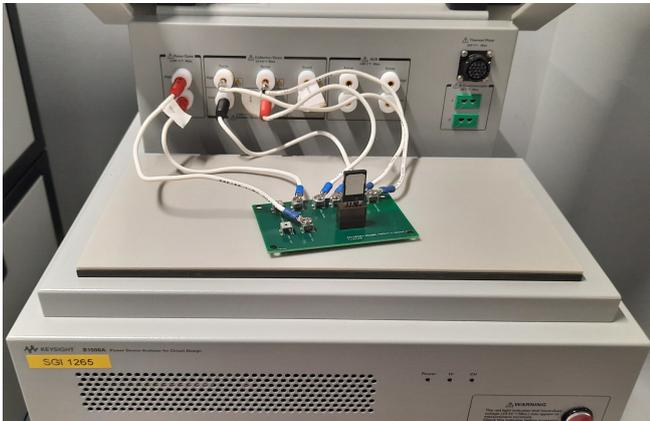
**Fig. 2:** Connection on the B1506A of a custom-built board for TO-247-4 packages
