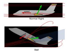
Fig. 2. Stall situation (source: Caliver, Wikimedia Commons)
