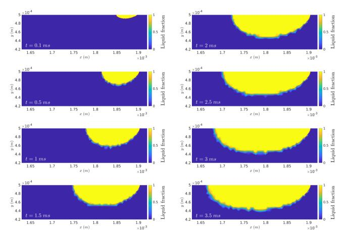
**FIGURE 8** Liquid fraction field at different instants over  $\mathcal{Z}$ .
