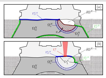
**FIGURE 5** Thermal modeling in the AF with in (a) an illustration of the global domain  $\Omega_G^N$  in dark grey and the overlap  $\Omega_o^N (= \Omega_c^N \cup \Omega_f^N)$ . In (b) an illustration of the local domain  $\Omega_L^N$  in light grey.
