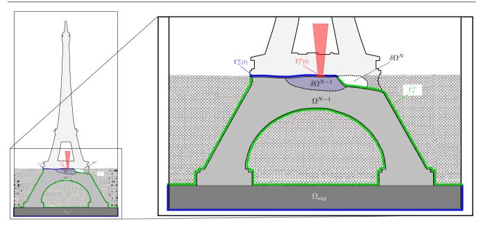
**FIGURE 3** A generic heat conduction problem over the domain  $\Omega^N = \Omega^{N-1} \cup \delta\Omega^{N-1}$  and the different parts of  $\partial\Omega^N$ .
