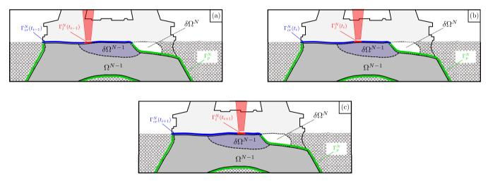
**FIGURE 4** Boundary conditions evolution: representation at times (a)  $t_{i-1}^N$ , (b)  $t_i^N$  and (c)  $t_{i+1}^N$  of the interval  $I_N$ .
