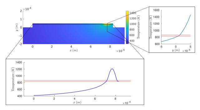
**FIGURE 25** Temperature distribution at 3.5 ms and its shape in a vertical and horizontal sectional view.
