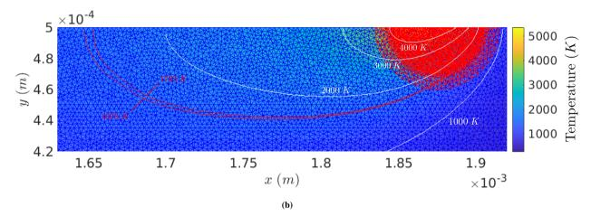
**FIGURE 11** Introduction of the Micro-Patch in red, the Meso-Patch in blue over the thermal field at 4 ms defined on  $\Omega$  in (a) and a zoom over  $\mathcal{Z}$  in (b). The set  $\mathcal{I}$  is represented in green in (a).
