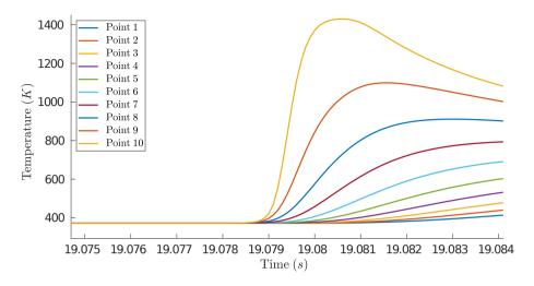
FIGURE 23 Temperature of the ten points during the last layer scan.
