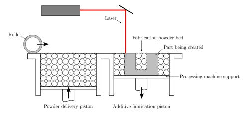
**FIGURE 1** Selective Laser Melting.
