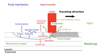
FIGURE 2 Illustration of physical phenomena in SLMP.
