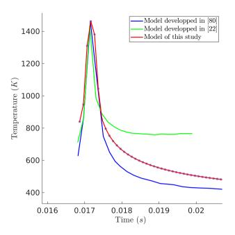
**FIGURE 24** Comparison of the temperature evolution at  $P_c$  over  $I_c$  we obtained with those of <sup>77</sup> and <sup>21</sup>.
