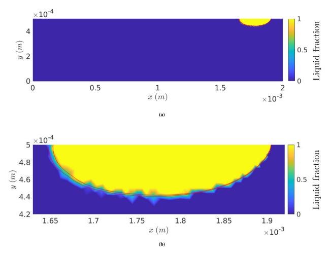
**FIGURE 10** Liquid fraction field at 4 ms over  $\Omega$  in (a) and over  $\mathcal{Z}$  in (b).
