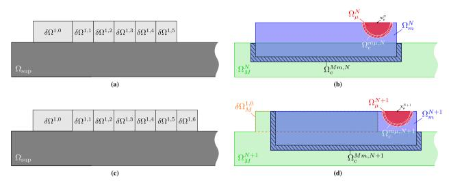
**FIGURE 17** Addition of the material increment  $\delta\Omega^{1,6}$  to the domain  $\Omega^6$ , represented in (a), to form the domain  $\Omega^7$ , represented in (c). The corresponding Arlequin three levels domains are illustrated in (b) and (d). In this illustration  $N^m_{\text{add}} = 6$ , so the transition from (b) to (d) corresponds to the passage, for the Meso-Patch, from its first layer last variable form to the fix one and the activation of the Macro-Block  $\delta\Omega^{1,0}_M$ .
