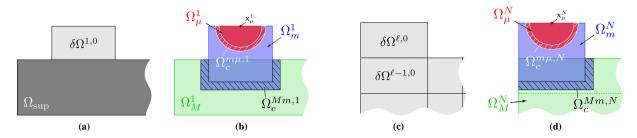
**FIGURE 16** Addition of the first material increment (i = 0) for the first layer  $(\ell = 1)$  in (a) and a  $\ell > 1$  layer in (c). The corresponding three-levels Arlequin domains are illustrated in (b) and (d).
