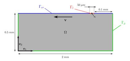
FIGURE 6 A representative two-dimensional model to identify the thermal scales.
