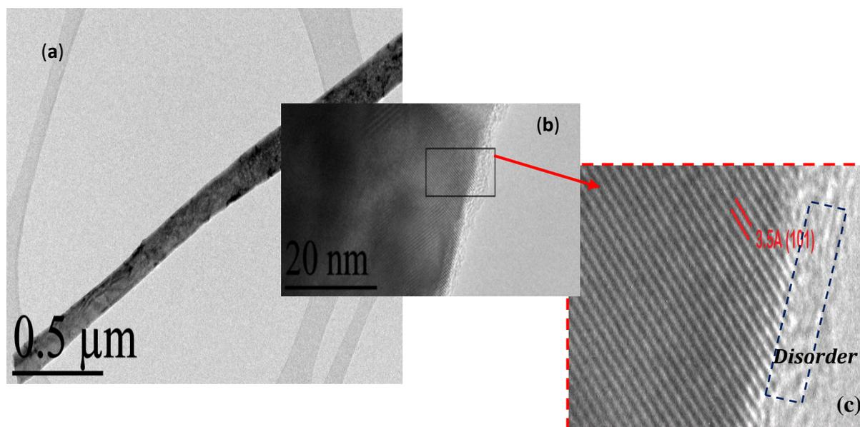
**Figure 5.** (a) Scanning transmission electron microscopy (STEM) of an individual H-TiO<sub>2</sub>/SiNW; HR-TEM micrographs at low (b) and high (c) resolution. The thickness of TiO<sub>2</sub> is 20 nm.
