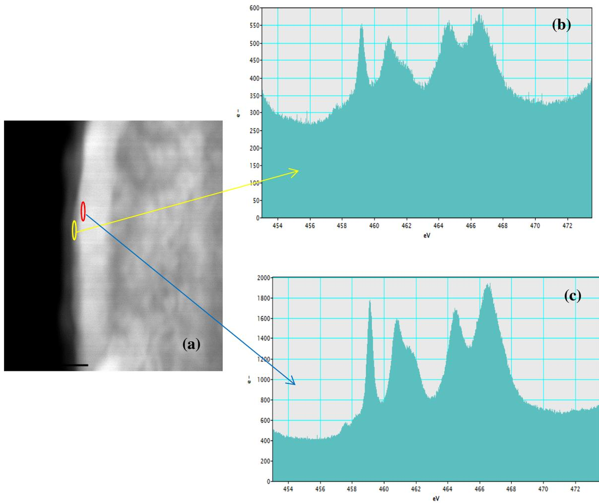
**Figure 6.** (a) STEM-HAADF image of TiO<sub>2</sub>/SiNW surface; EELS spectra of (b) the extreme surface (less than 3 nm) and (c) 15 nm below the surface of TiO<sub>2</sub>.
