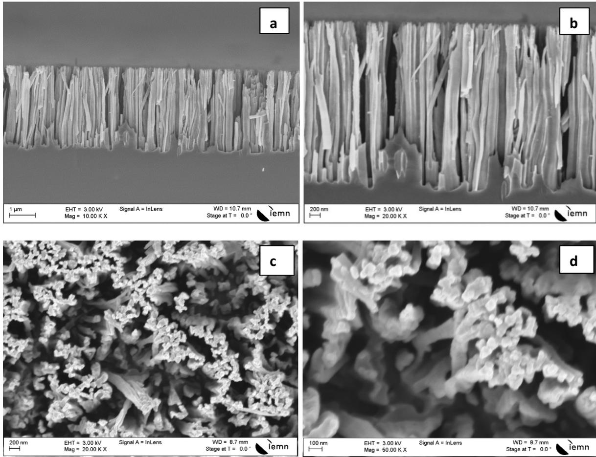
**Figure 1:** Cross-section (a,b) and top-view (c,d) SEM micrographs of SiNW arrays coated with 20 nm of TiO<sub>2</sub> by ALD.
