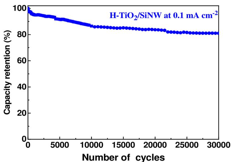
**Figure 11.** Life time testing of the H-TiO<sub>2</sub>/SiNW electrode in an aqueous 1M Na<sub>2</sub>SO<sub>4</sub> electrolyte.
