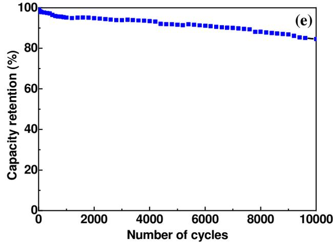
**Figure 12.** (a) CV curves of H-TiO<sub>2</sub>/SiNW symmetric electrochemical cell collected at various scan rates (potential window: -0.4 to +0.3 V), (b) GCD profiles of the device charged at 0.5 mA cm<sup>-2</sup>, (c) specific capacitance *versus* scan rate, (d) Ragone plot, (e) Capacitance retention percentage of the H-TiO<sub>2</sub>/SiNW symmetric electrochemical supercapacitor for 10,000 cycles at 0.5 mA cm<sup>-2</sup>.
