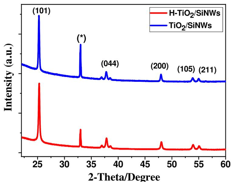
**Figure 2.** X-ray diffractograms of TiO<sub>2</sub>/SiNW and H-TiO<sub>2</sub>/SiNW samples.
