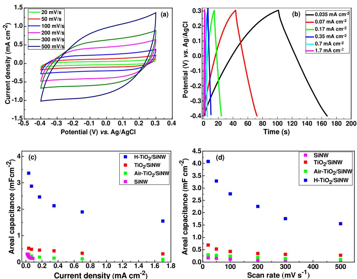
**Figure 9.** (a) CV plots of H- $\text{TiO}_2/\text{SiNW}$  acquired at different scan rates (potential range: -0.4 to +0.3 V), (b) GCD plots recorded for H- $\text{TiO}_2/\text{SiNW}$  at different current densities, (c) Areal capacitance of all electrodes *versus* scan rate, (d) Areal capacitance of all electrodes *versus* current density.
