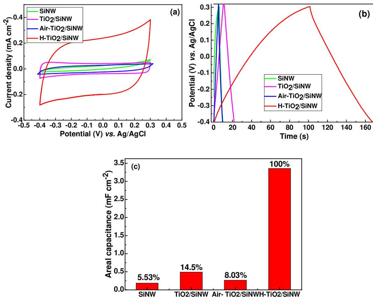
**Figure 8.** (a) CV plots of different electrodes collected at  $100 \text{ mV s}^{-1}$  in a potential range from -0.4 to +0.3V, (b) GCD profiles recorded at  $0.035 \text{ mA cm}^{-2}$ , (c) Areal capacitance of different electrodes acquired at  $100 \text{ mV s}^{-1}$ .
