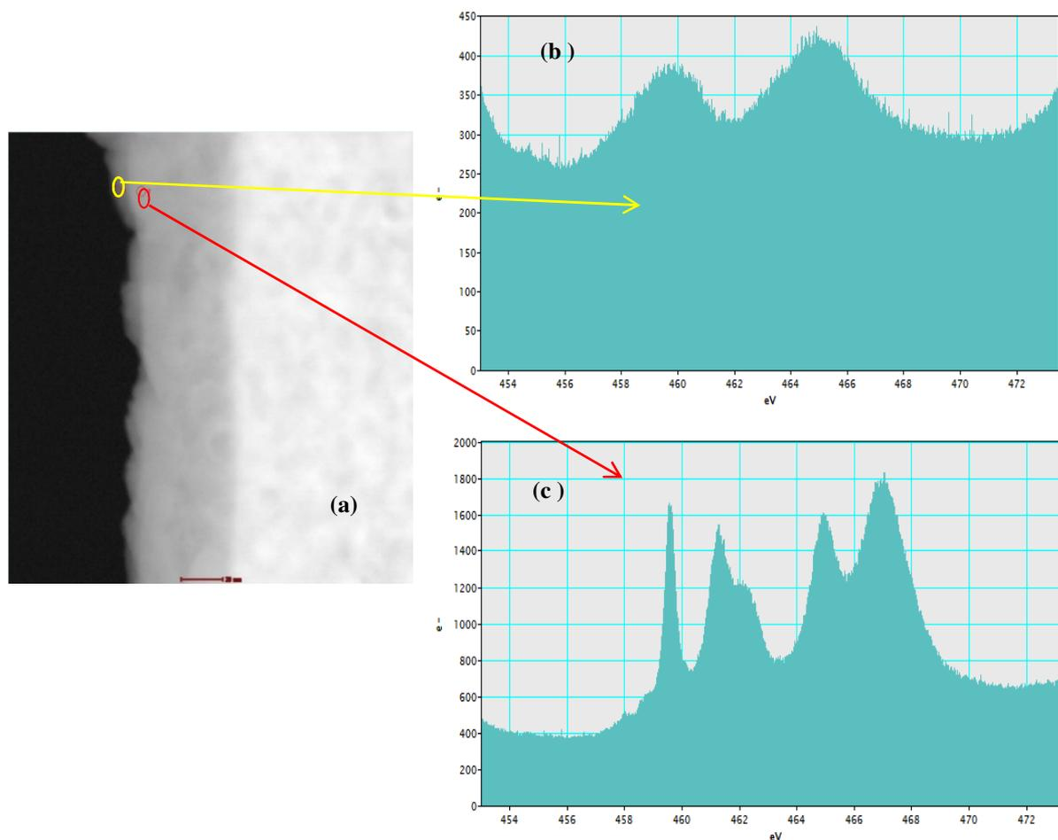
**Figure 7.** (a) STEM-HAADF image of H-TiO<sub>2</sub>/SiNW surface; EELS spectra of (a) extreme surface (less than 3 nm) ~~Ti reduced~~ and (c) 15 nm below the surface of TiO<sub>2</sub>.
