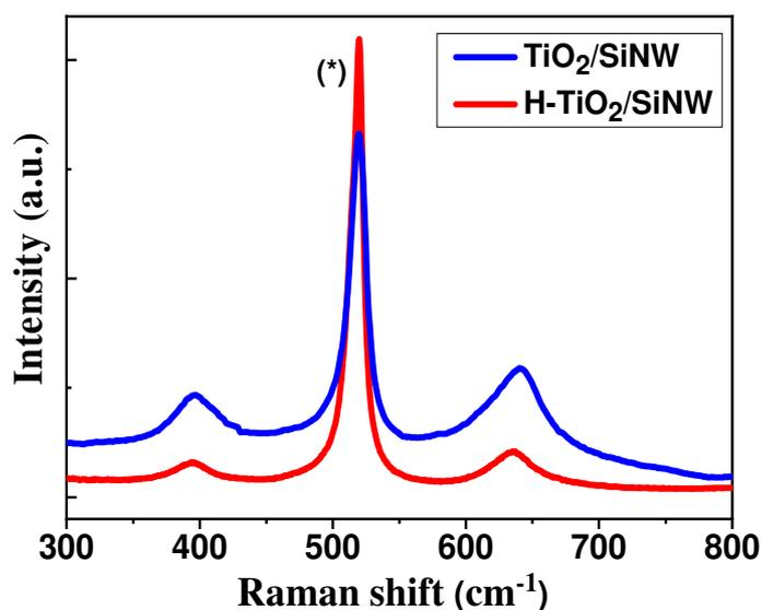
**Figure 3.** Raman plots of TiO<sub>2</sub>/SiNW (blue) and H-TiO<sub>2</sub>/SiNW (red) samples.
