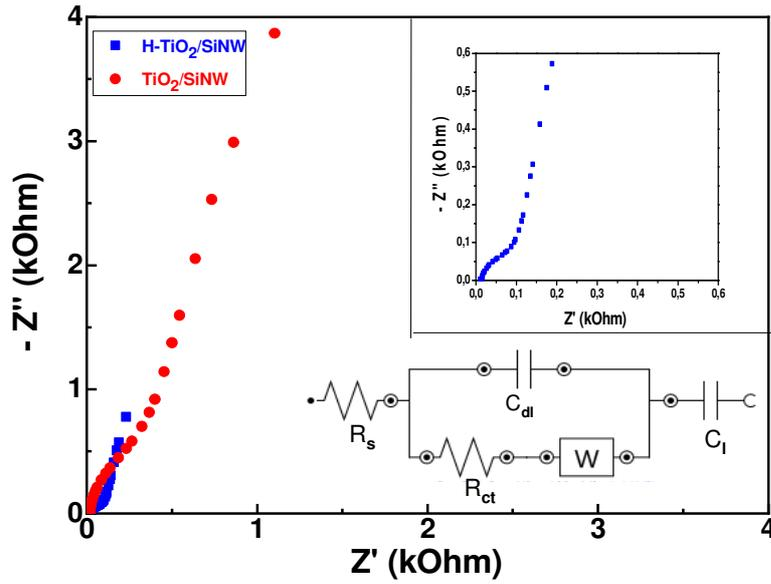
**Figure 10.** Nyquist plot in the 0.1 Hz to  $5 \times 10^5$  Hz frequency range. Inset displays the enlarged region at high frequency for H-TiO<sub>2</sub>/SiNW electrode.
