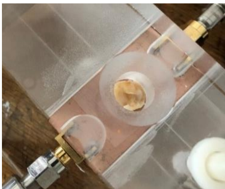
Figure 8. Sample holder setup with an atheromatous plaque
