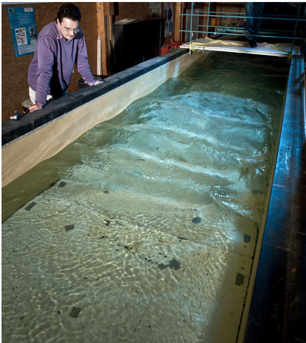
FIG. 3. Wave blocking at a dispersive group velocity horizon in the 2010 Nice experiments [24] (see also Figure 1 of [21] reporting a similar picture about the 2008 experiments [2]): the short waves correspond mainly to the blue-shifted modes B^\omega at the dispersive horizon or wave blocking line (if amplified by the simultaneous appearance of negative modes N^\omega , they would correspond to stimulated Hawking radiation) and which are converted from the long incoming modes I^\omega . In the near horizon region where k_I^\omega \simeq k_B^\omega one observe sometimes partial wave breaking and parasitic capillary waves conversion on the front wave. Picture by Olivier Monge, Agence MYOP.
