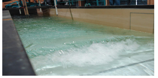
FIG. 25. The turbulent hydraulic jump in the original setup of the Nice 2008 experiments [2] at high Froude numbers seen downstream just after the flat part of the obstacle whose boundary corresponds to the inclined grey band in the lower part of the image. The wave-maker with its cyan painting is located in the background of the picture: the flow points towards the picture from the lower right corner to the upper left corner. This transcritical regime was replaced by a subcritical one with a slower speed and an almost flat free surface or with a small depression in order to propagate counter-current waves on a smoother free surface from downstream the bottom obstacle.
