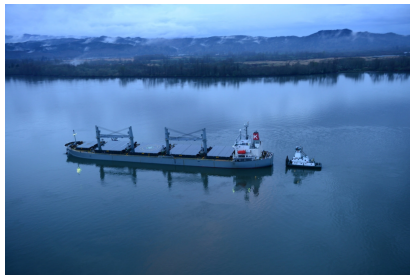
The motor vessel Sparna lists to its port side after taking on water in void spaces after running aground while transiting the Columbia River, 2016. U.S. Coast Guard Photo
