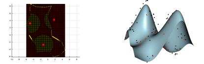
Approximation of the Loire surface covered by one antenna for varying locations,  $S(x_1, x_2)$ . The approximation (silver surface) is the mean of a kriging model learned from 20 examples (the red bullets). The black bullets are test points (not learned), providing some insights into the imperfections of the approximation.
