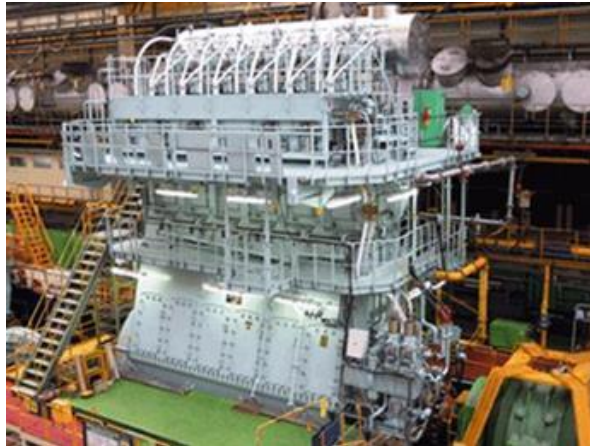
Figure 9. A large ship engine (Wärtsilä X62 engine), the steps on the left side can be used for an estimate of the scale. ( https://www.wartsila.com/media/news/08-01-2015-wartsila-x62-engine-now-fully-approved-and-available-to-the-market )
