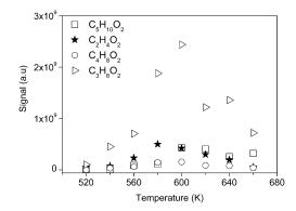
**Fig. 8.** Comparison between  $C_2$ ,  $C_3$ ,  $C_4$  and  $C_5$  alkenyl hydroperoxides formed during the low temperature oxidation of n-pentane.  $C_2$ ,  $C_3$  and  $C_4$  alkenyl hydroperoxides profiles were obtained using  $C_{18}$  UHPLC APCI(–)-HRMS (m/z 59.0139, 73.0295, and 87.0452 respectively). The  $C_5$  profile was acquired by UHPLC APCI(+)-HRMS (m/z 103.0750). Experimental errors are estimated to be ~ 40%.
