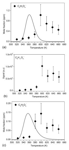
**Fig. 15.** Formation of HOMs  $C_5H_8O_4$ ,  $C_5H_{12}O_4$ , and  $C_5H_{10}O_4$  produced during the low temperature oxidation of n-pentane. Comparison between experimental results (symbols) using FIA APCI(–)-HRMS ( $C_5H_7O_4^-$  at m/z 131.0350,  $C_5H_{11}O_4^-$  at m/z 135.0663, and  $C_5H_9O_4^-$  at m/z 133.0506) and modeling data (line) for  $C_5H_{10}O_4$ , and  $C_5H_8O_4$ ). Experimental data were scaled to simulated results. HRMS errors are estimated to be ~ 40%.
