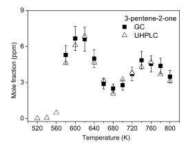
**Fig. 13.** Comparison of 3-pentene-2-one mole fraction profiles obtained after  $C_{18}$  UHPLC- APCI(+)-HRMS ( $C_5H_9O^+$ , m/z 85.0647) and GC-FID analyses. UHPLC data were scaled to those obtained in GC. Results could not be compared with computation profiles because these molecules are not present in the WS kinetic model.
