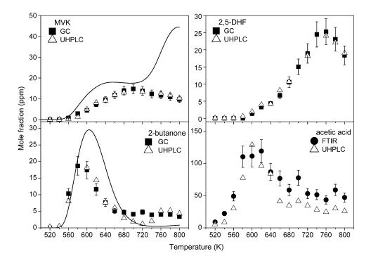
**Fig. 3.** Formation of MVK, 2,5-DHF, 2-butanone (APCI(+)-HRMS) and, acetic acid (APCI(-)-HRMS) during the oxidation of 2500 ppm of n-pentane at 10 atm. C<sub>18</sub> UHPLC analysis results were scaled to GC and FTIR results (data: symbols, WS model: lines).
