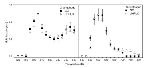
**Fig. 12.** Comparison between 2-pentanone and 3-pentanone mole fraction profiles obtained by  $C_{18}$  UHPLC APCI(+)-HRMS ( $C_5H_{11}O^+$ , m/z 87.0802) and GC analyses. UHPLC results were scaled to GC data. Results could not be compared with simulated profiles because these molecules are not present in the WS kinetic model.
