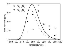
**Fig. 9.** Evolution of  $C_3H_5O_3^-$  (m/z 89.0245),  $C_4H_7O_3^-$  (m/z 103.0401) profiles corresponding to ketohydroperoxides  $C_3H_6O_3$ , and  $C_4H_8O_3$  formed during the oxidation of n-pentane in JSR at 10 atm. Experimental data (Symbols) were scaled to modeling results (continuous line for  $C_3H_6O_3$  and dotted line for  $C_4H_8O_3$ ). Experimental results were obtained using a Silica HPLC column and APCI(–)-HRMS. HRMS errors are estimated to be ~ 40%.
