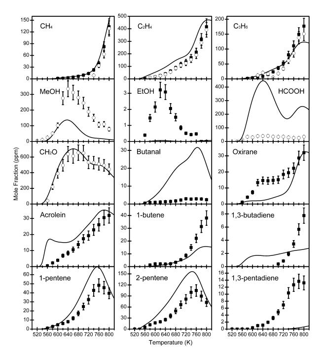
**Fig. 2.** Comparison between experimental mole fraction of organic species and simulations (using the WS model) for the oxidation of 2500 ppm of n-pentane in JSR at a pressure of 10 atm, ( $\phi$  = 0.5, residence time of 1.5 s). Symbols: data obtained by GC-FID (square) and FTIR (circle).
