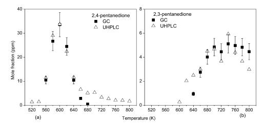
**Fig. 14**. Comparison between 2,4-pentanedione (a) and 2,3-pentanedione (b) mole fractions obtained by GC-FID and UHPLC- APCI(+)-HRMS ( $C_5H_9O_2^+$ , m/z 101.0593). UHPLC data were scaled to GC-FID data. Results could not be compared with simulations because these molecules are not included in the WS kinetic model.
