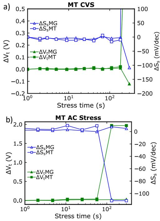
Fig. 8. a) CVS and b) AC stress dependence of  $V_t$  and  $S_s$  shift as function of stress time for MT gate stress with  $V_{g,MT} = 8$  V,  $V_{d,s,b} = 0$  V.
