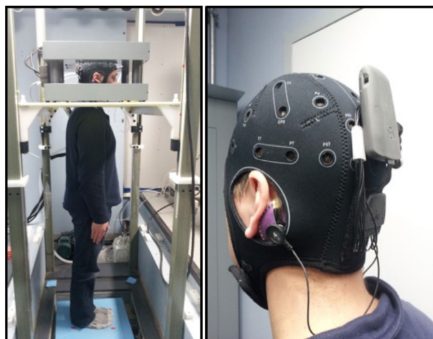
FIGURE 1. Stimulation apparatus. Volunteers stood in complete darkness, feet together, arms by their side and eye closed on a 1.5 cm foam pad covering the force plate. Their head was fully stimulated by Helmholtz-like coils centered on their ears, with ELF-MF stimulations at 8.89 T/s, 26.66 T/s and 39.98 T/s (left panel). The binaural bipolar DC montage stimulating both vestibular systems at 2 mA. The cathode is behind the right mastoid process and the anode is behind the left mastoid process (right panel).
