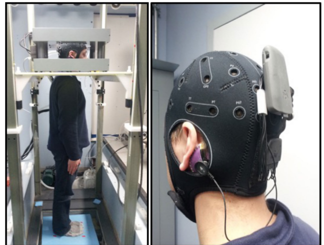
FIGURE 1. Stimulation apparatus. Volunteers stood in complete darkness, feet together, arms by their side and eye closed on a 1.5 cm foam pad covering the force plate. Their head was fully stimulated by Helmholtz-like coils centered on their ears, with ELF-MF stimulations at 8.89 T/s, 26.66 T/s and 39.98 T/s (left panel). The binaural bipolar DC montage stimulating both vestibular systems at 2 mA. The cathode is behind the right mastoid process and the anode is behind the left mastoid process (right panel).
