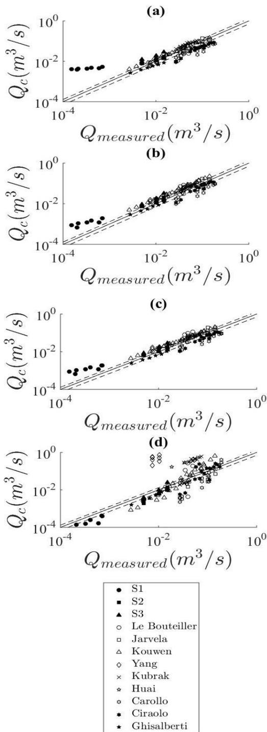
**Fig. 6.** Comparison of the total discharge over vegetated bed for the model of Huthoff (a), the Meijer and Van Velzen (b), Cassan and Laurens (c), and Rubol *et al.* (d) ( $C_d = 1$  for all experiments). Experiments from (Le Bouteiller and Venditti, 2015; Jarvela, 2005; Kouwen and Unny, 1969; Yang and Choi, 2009; Kubrak *et al.*, 2008; Huai *et al.*, 2009; Carollo, Ferro, Termini, 2002; Ciraolo, Ferreri, 2007; Ghisalberti and Nepf, 2006). Dash lines represents a deviation of 30 %.
