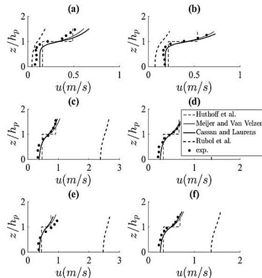
**Fig. 4. Comparison of velocity profiles of (Kubrak *et al.*, 2008) experiments and the 4 models. The figures correspond respectively to the experiments 1.1.3 (a), 1.2.1 (b), 2.2.1 (c), 3.1.1 (d), 3.2.1 (e), 4.1.1 (f), 4.2.1 (g).**
