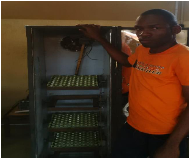
Figure 2: View of the Egg Incubator during Construction
