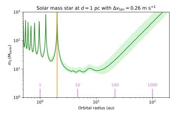
**Fig. 1.** Sensitivity function  $m_2 = f(r)$  for a solar mass star at a distance of 1 pc. The pink markings show a selection of orbital periods in years, and the orbital radius corresponding to an orbital period equal to the *Gaia* EDR3 duration (34 months) is displayed as an orange vertical line.
