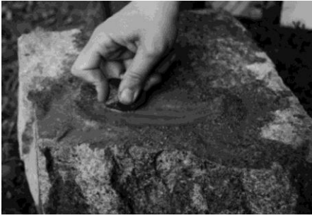
Fig. 4. Experimental protocol applied for polishing diasporite celts. Only abrasives vary.
