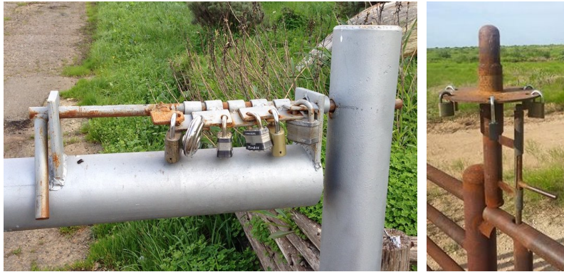
Fig. 2. Two ad-hoc physical 1-out-of-6 padlocks.
