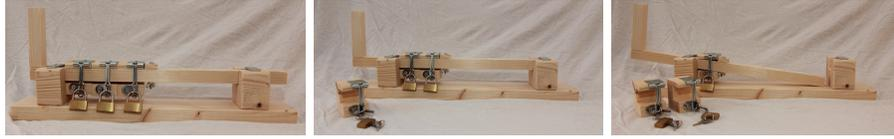
Figure 6: Physical 2-out-of-3 lock. **Left:** all three blocks attached, lock closed. **Middle:** one block removed, the bar can be moved to the left, but not sufficiently far to open. **Right:** two locks are removed, the barrier is open.
