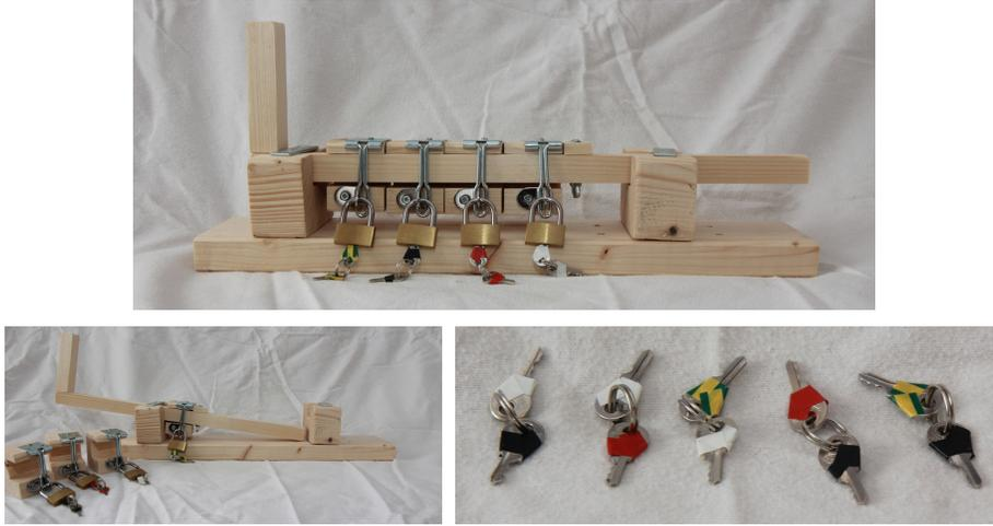
Figure 9: Physical 3-out-of-4 threshold padlock system. **Top:** all locks closed. **Left bottom:** device opened using 3 out of the 4 locks. **Right bottom:** Example key distribution to achieve a 2-out-of-5 threshold system using only 4 padlocks and the 3-out-of-4 device above (see Section 4.2, Algorithm 1 and Theorem 10).
