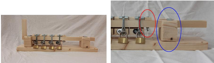
Figure 8: **Left:** Physical 2-out-of-4 threshold padlock system; **Right:** configuring our prototype: the block in the red circle fixes the number  $n$  (here: 4), the block in the blue circle fixes the threshold  $k$  (here: 3). One can also see the holes that allow the block to be fixed in other positions.
