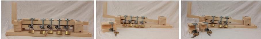
Figure 7: Physical lock with weighted keys. **Left:** all blocks are attached and locked. **Middle:** the “master” key was used to open the larger block, unlocking the barrier. **Right:** two “normal” keys opening normal blocks also allow to open the barrier.
