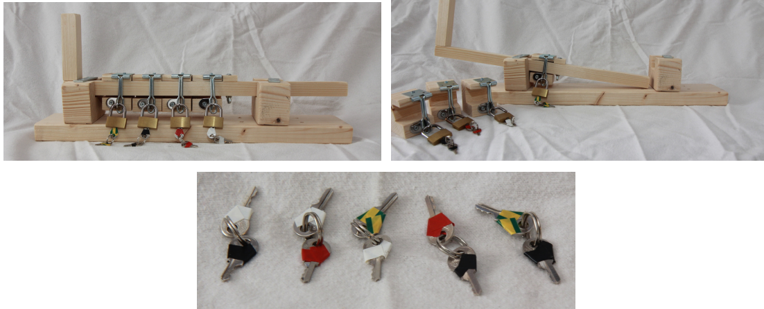
Fig. 9. Physical 3-out-of-4 threshold padlock system. Left: all locks closed. Right: device opened using 3 out of the 4 locks. Bottom: Example key distribution to achieve a 2-out-of-5 threshold system using only 4 padlocks and the 3-out-of-4 device.
