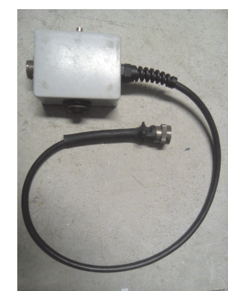
Signal injector module:
