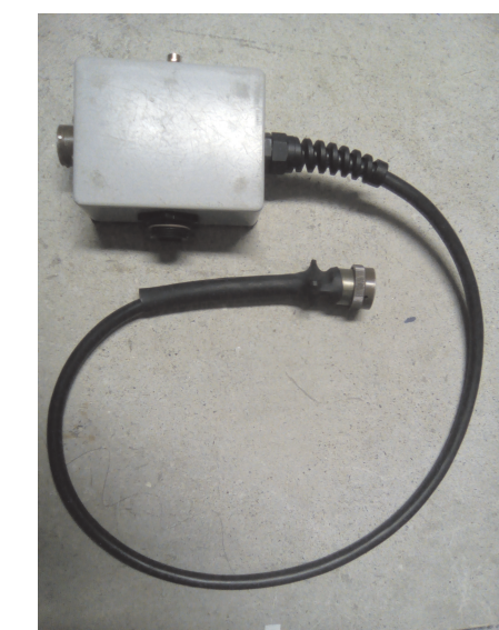
Signal injector module:
