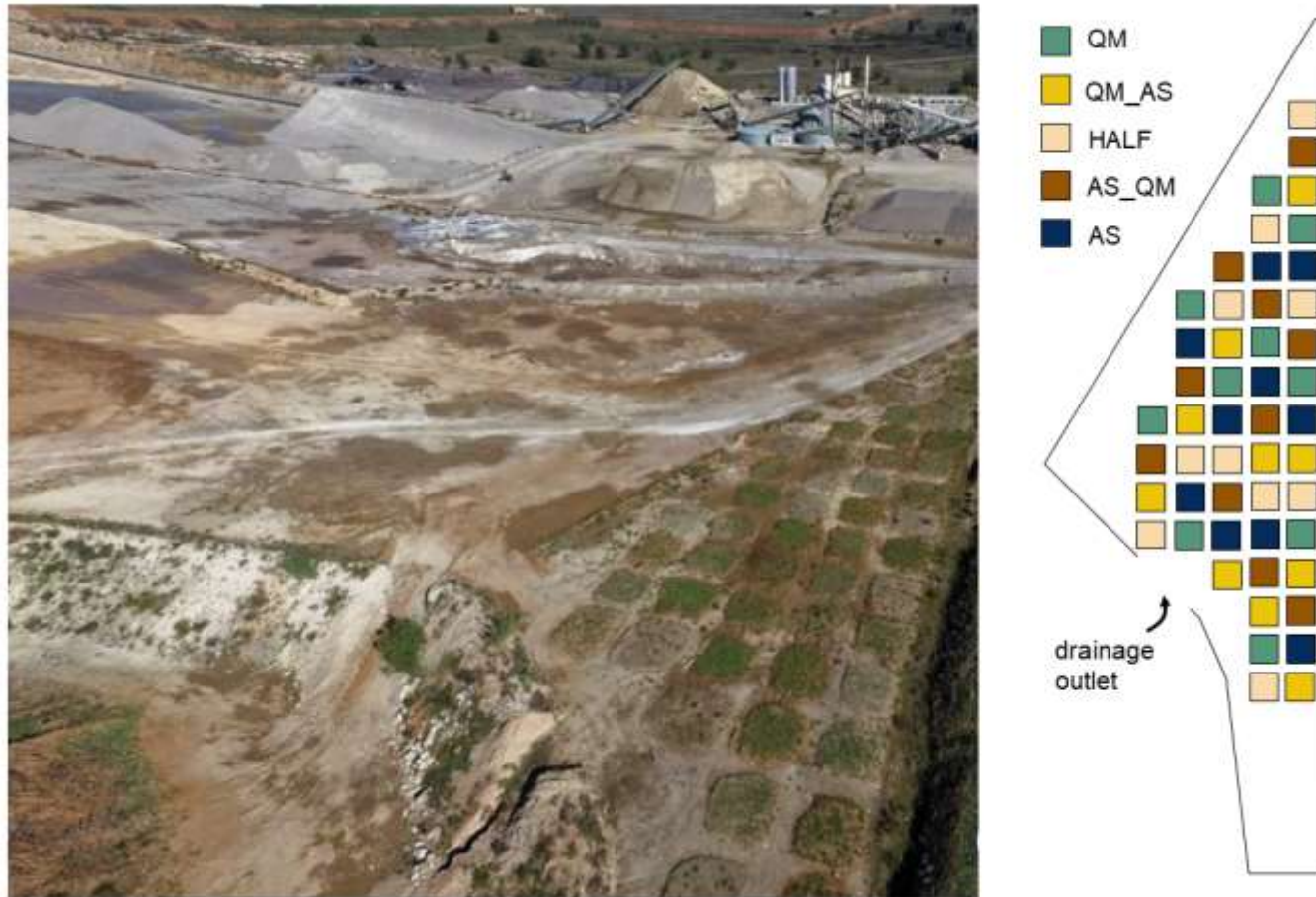
Figure C. Experimental plots set up in the Ménéudelle quarry in 2016 (50 plots \times 5 mixtures (QM: 100% of raw Quarry Material; QM_AS: 75% of raw Quarry Material and 25% of Arable Soil; HALF: 50% of each; AS_QM: 75% of Arable Soil and 25% of raw Quarry Material; AS: 100% of Arable Soil) \times 2 sowing treatments + a drainage outlet) Photography: SCLM
