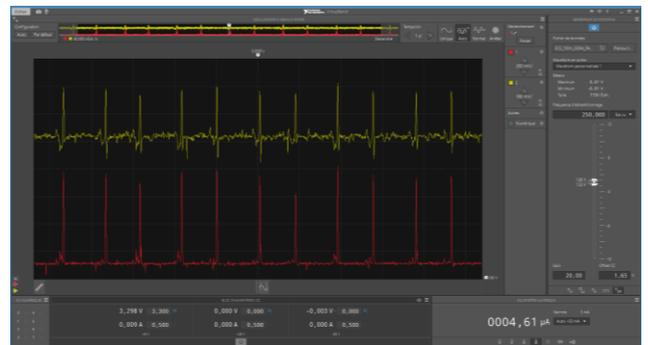
Fig. 16. Measurement results of the analog square function output (channel 1 in red; Y-axis scale = 200mV/div) when pulses synchronized with heartbeats in electrocardiogram occur on  $V_{IN}$  (channel 2 in yellow; Y-axis scale = 100mV/div). X-axis scale is equal to 1s/div.
