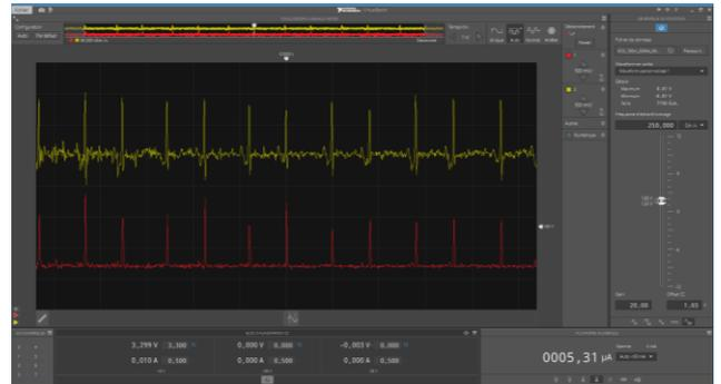
Fig. 15. Measurement results of the TEO output  $V_{OUT}$  (channel 1 in red) when pulses synchronized with heartbeats in electrocardiogram occur on  $V_{IN}$  (channel 2 in yellow). Y-axis scale is equal to 100 mV/div for both channels and x-axis scale is equal to 1 s/div.
