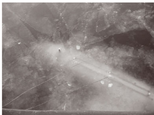
Fig. 3. Autosub surfacing in light sea-ice cover. Note the possibility of damage to antennae protruding from the vehicle.
