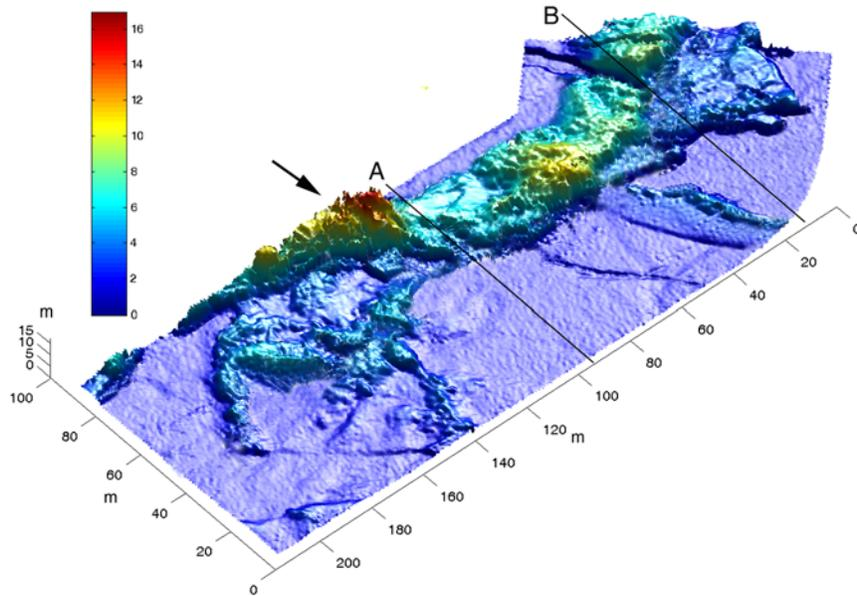
**Figure 4.** The main study ridge. The plot is displayed without vertical exaggeration, and shows the very steep topography of this young ridge. Maximum draft in the swath is 16.8 m, and the AUV was running at 25 m depth. The dappled character of the FY ice evident in this backlit image arises from the  $\pm 3$  cm standard error in individual bins.
