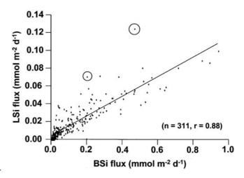
**Figure 8.** Linear correlation between BSi and LSi fluxes. The two circled data points correspond to samples with high LSi level as compared to BSi (see text for details).
