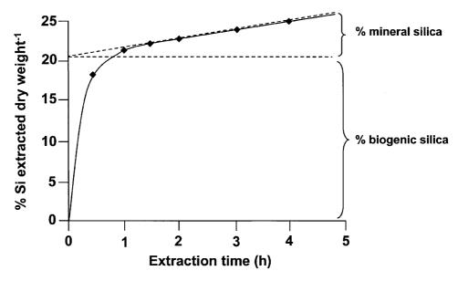
**Figure 2.** Kinetics of silica extraction versus time. The first part of the curve mainly corresponds to rapid BSi dissolution, whereas the second, linear one corresponds to slower LSi dissolution. The biogenic silica content of the sample is estimated by linear extrapolation at time zero intercept.
