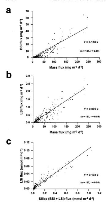
**Figure 6.** (a) BSi fluxes versus mass fluxes, (b) LSi fluxes *versus* mass fluxes, and (c) LSi fluxes versus total silica (BSi + LSi) fluxes from February 2001 to February 2002 (bulk data). Data from southwest sediment traps and 400 m northwest sediment traps were excluded from the relationships because records have been interrupted on the annual cycle due to logistical problems.
