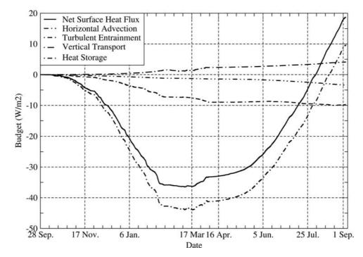
**Figure 11.** Annual evolution of the cumulative domain-averaged mixed layer heat budget. Units are in W  $m^{-2}$ , obtained by dividing each term of the mixed layer heat budget by the total cumulative time (343 days).
