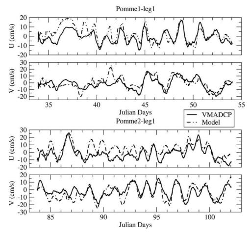
**Figure 8.** Comparison of vessel-mounted acoustic Doppler current profiler (VMADCP) measurements (averaged over the first 100 m below the surface) with simulated surface currents (cm s<sup>-1</sup>) along the ship trajectory.
