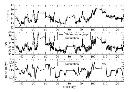
**Figure 6.** Comparison of the thermosalinograph measurements with the simulated SST (°C) and SSS (psu) along the ship trajectory. The simulated dynamic height (mdyn) along the ship trajectory is presented to show the correlation between Hdyn with the SSTs and SSSs.
