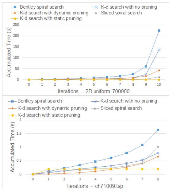
Figure 12: Accumulated time of Find Min 1 with different NNS algorithms in different iterations to build EMST for 2D uniform-700000 and ch71009.tsp benchmarks.
