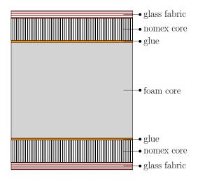
Figure 10: Sketch of triple-core sandwich stack.
