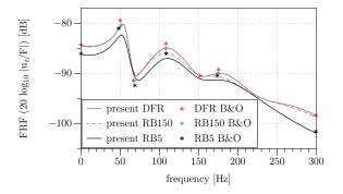
Figure 7: Frequency response function of  $P(x, y) = (L_1/4, L_2/4)$  of the SSSS sandwich plate with ISD112 core: Direct Frequency Response (DFR) and FR obtained from a real basis with 5 and 150 modes.
