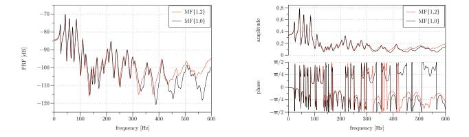
Figure 13: FRF of the triple-core panel (left) and related amplitude and phase diagrams (right): comparison of MF{1,2} and MF{1,0} models.
