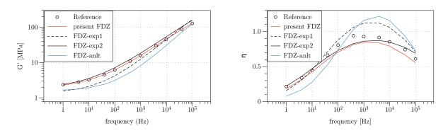
Figure 2: Frequency-dependent storage modulus (left) and loss factor (right) for Deltane 350: Reference curves and FDZ models.
