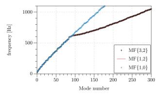
Figure 11: First 300 natural frequencies of the CCCC triple-core panel for 3 models for the melamine foam core.
