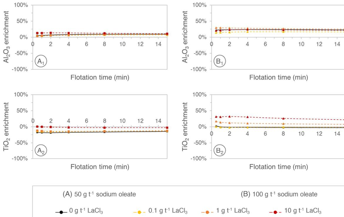
Figure 11: Influence of the addition of pre-mixed  $\text{LaCl}_3$  and sodium oleate on the cumulative  $\text{TiO}_2$  and  $\text{Al}_2\text{O}_3$  enrichment of the floated product (enrichment over feed material).
