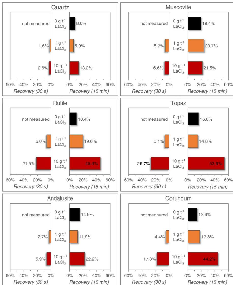
Figure 7: Cumulative recovery of main gangue minerals after 30 s and 15 min of flotation using a  $100 \text{ g t}^{-1}$  collector dosage. These results are based on the MLA measurements of the flotation feed material, the flotation products collected after 30s and the non-floated products collected after 15 min of flotation.
