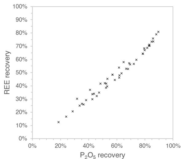
Figure 5: Correlation between REE and  $\text{P}_2\text{O}_5$  recovery during the flotation.
