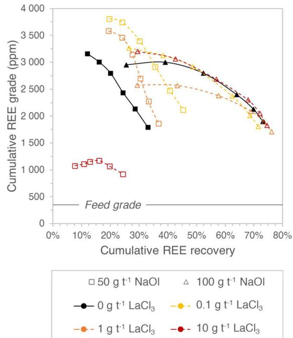
Figure 10: Influence of the addition of pre-mixed LaCl<sub>3</sub> and sodium oleate (NaOl) on the progress of REE recovery and concentrate REE grade during flotation.
