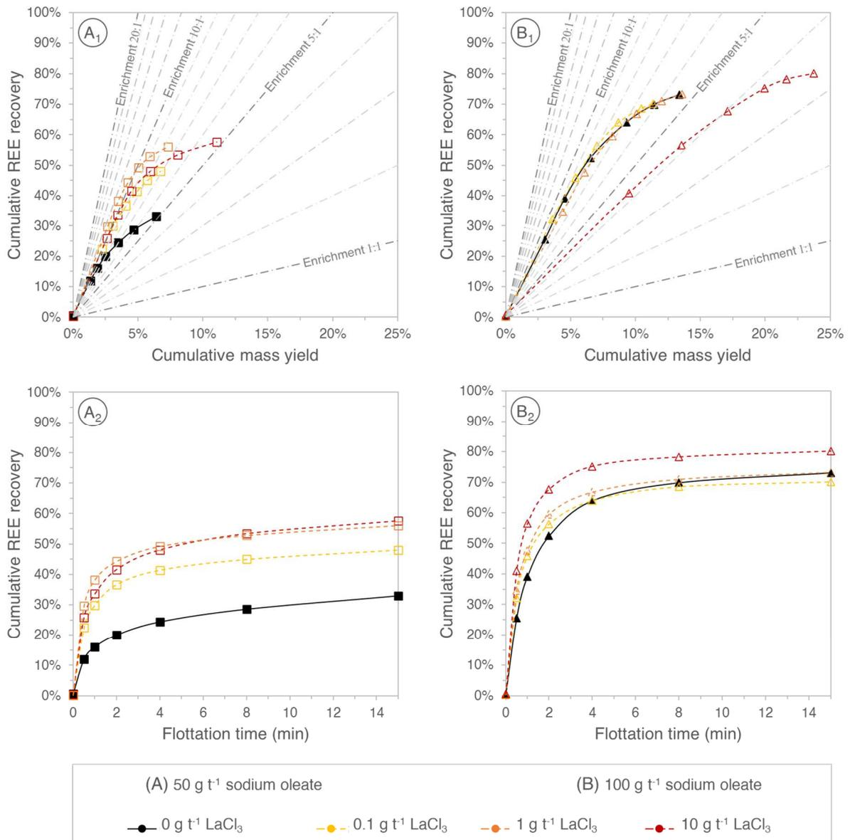
Figure 3: Influence of the sequential addition of LaCl<sub>3</sub> and sodium oleate on the progress of REE recovery and yield during flotation.
