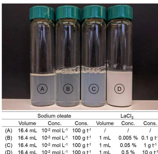
Figure 8: Mixed sodium oleate /  $\text{LaCl}_3$  solutions before addition to the flotation cell. “conc” are the concentrations of the individual solutions before mixing and “cons” are the equivalent reagents consumptions for 500 g of material treated.
