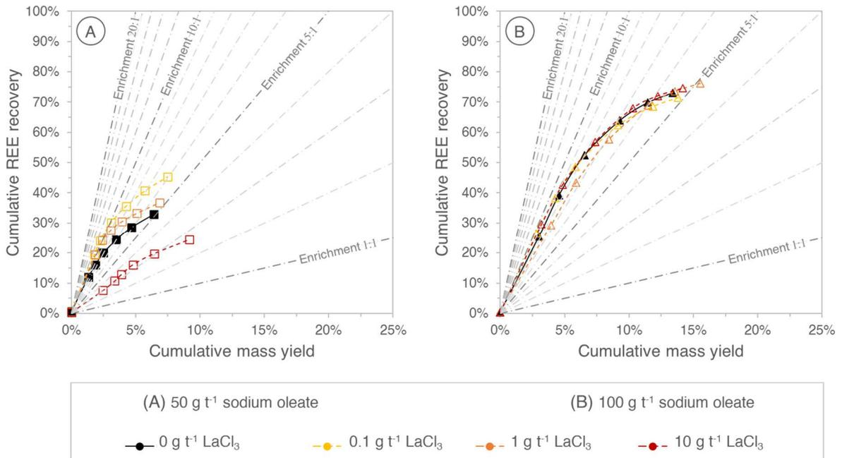
Figure 9: Influence of the addition of pre-mixed LaCl<sub>3</sub> and sodium oleate on the progress of REE recovery and yield during flotation.
