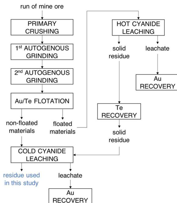
Figure 1: Gold and tellurium extractive metallurgy operations.
