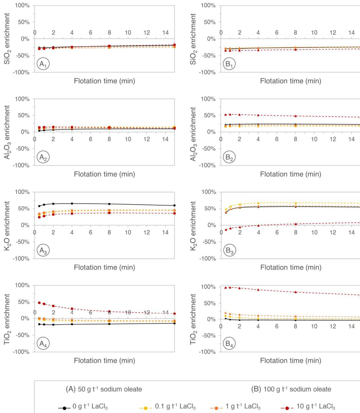
Figure 6: Influence of the sequential addition of  $\text{LaCl}_3$  and sodium oleate on the cumulative  $\text{TiO}_2$ ,  $\text{SiO}_2$ ,  $\text{Al}_2\text{O}_3$ , and  $\text{K}_2\text{O}$  enrichment in the floated products. The (cumulative) enrichment is obtained by dividing the (cumulative) grade of the floated product on the grade of the feed material.
