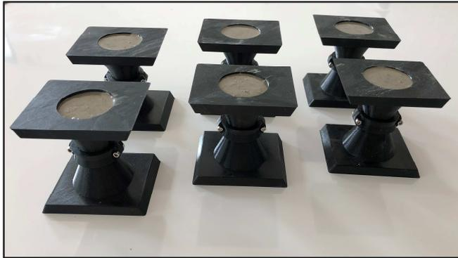
**Figure 15** Exchangeable part of Double Dumbbell device filled with mortar at rest before tensile strength measurements.
