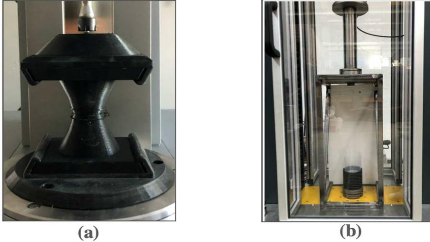
**Figure 2** Devices used to characterize tensile behavior of cement-based materials -
