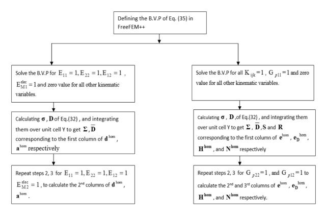
Fig.3: Schematic diagram for computing the effective dhom, ahom, ehom, eDhom, Hhom, Nhom matrices
