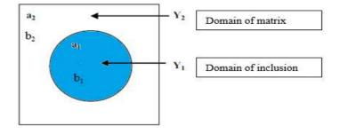
**Fig.1:** Two elastic materials with rigidity and piezoelectric coefficients  $a_i$ ,  $b_i$  (the index i stands for the constituent within the unit cell)
