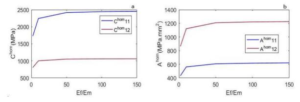
**Fig.12:** Variation of the first gradient rigidity coefficients (a), and second gradient rigidity coefficients (b) versus the ratio of fiber to matrix Young moduli Ef/Em.
