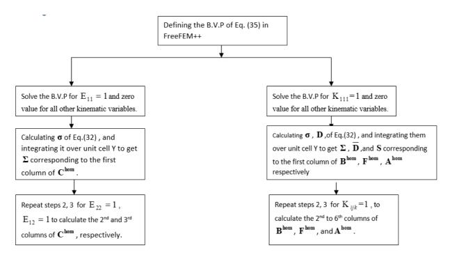
Fig.2: Schematic diagram for the computation of the effective moduli Chom, Bhom, Fhom, Ahom
