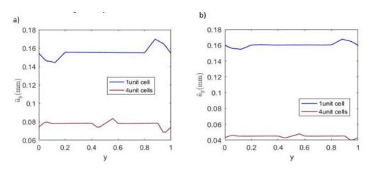
**Fig.16:** Distribution of the fluctuating displacement  $\tilde{u}_y$  (in mm), due to the macroscopic strain component  $E_{11} = 1$ , and b) strain gradient component  $K_{111} = 1$  along a vertical line through the centers of the inclusions for the pure elastic medium with no electric effects.
