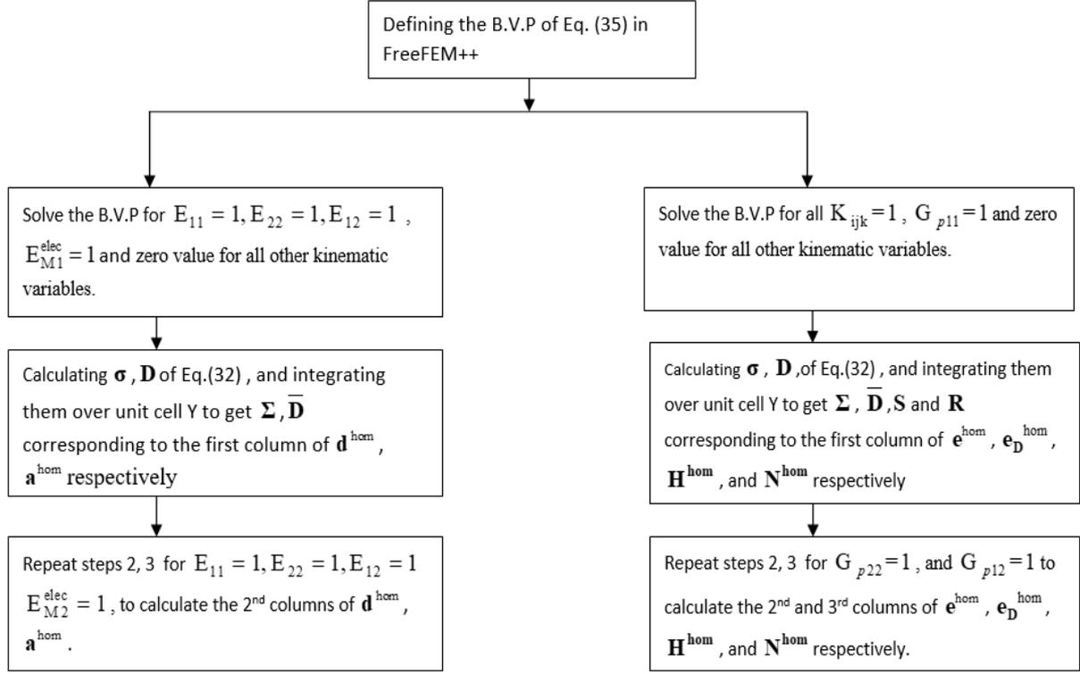
**Fig.3:** Schematic diagram for computing the effective  $\mathbf{d}^{\text{hom}}$ ,  $\mathbf{a}^{\text{hom}}$ ,  $\mathbf{e}^{\text{hom}}$ ,  $\mathbf{eD}^{\text{hom}}$ ,  $\mathbf{H}^{\text{hom}}$ ,  $\mathbf{N}^{\text{hom}}$  matrices
