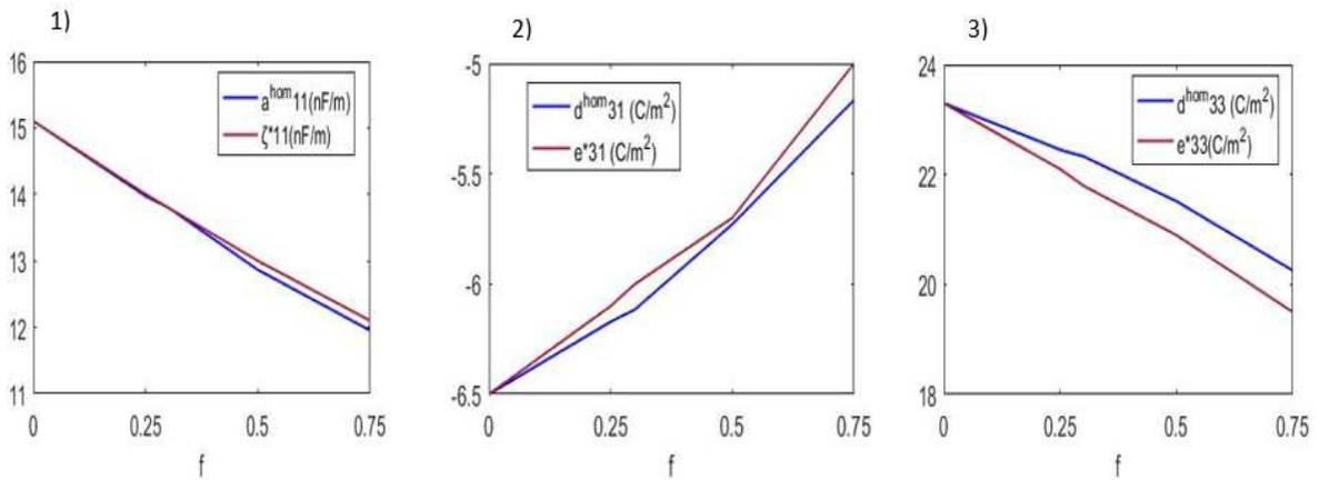
**Fig. B:** Variation of the 1) dielectric coefficient, 2) and 3) piezoelectric coefficients as a function of the volume fraction. Red corresponds to the results in (Sevostianov, I et al. 2007), blue corresponds to the results using the variational approach.
