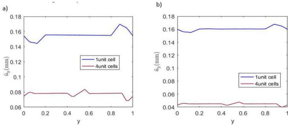
**Fig.16:** Distribution of the fluctuating displacement  $\tilde{u}_y$  (in mm), due to the macroscopic strain component  $E_{11} = 1$ , and b) strain gradient component  $K_{111} = 1$  along a vertical line through the centers of the inclusions for the pure elastic medium with no electric effects.
