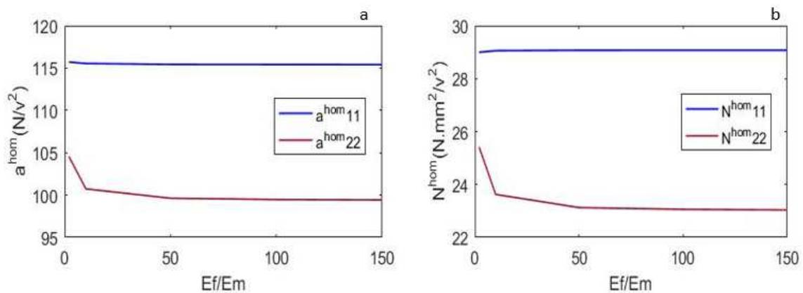
**Fig.13:** Variation of the permittivity coefficients (a), and coefficients of  $N^{hom}$  matrix (b) versus the ratio of fiber to matrix Young moduli  $E_f/E_m$ .
