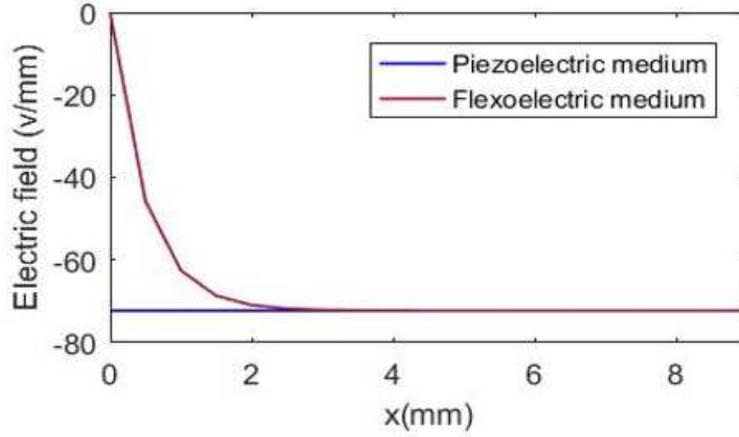
**Fig.5:** Electric field with and without flexoelectric term under a constant applied stress  $\Sigma_0$ .
