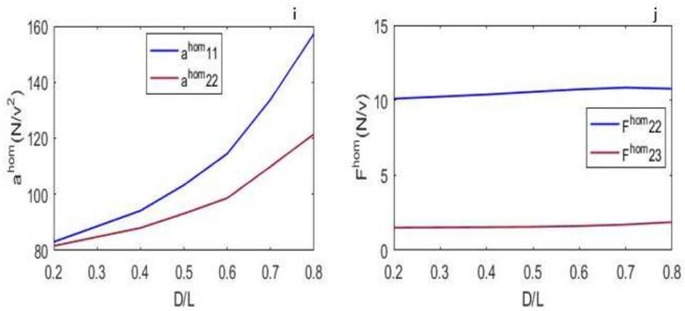
**Fig.11:** Homogenized i) permittivity coefficients  $a^{\text{hom}}$ , j) coupling coefficients  $F^{\text{hom}}$
