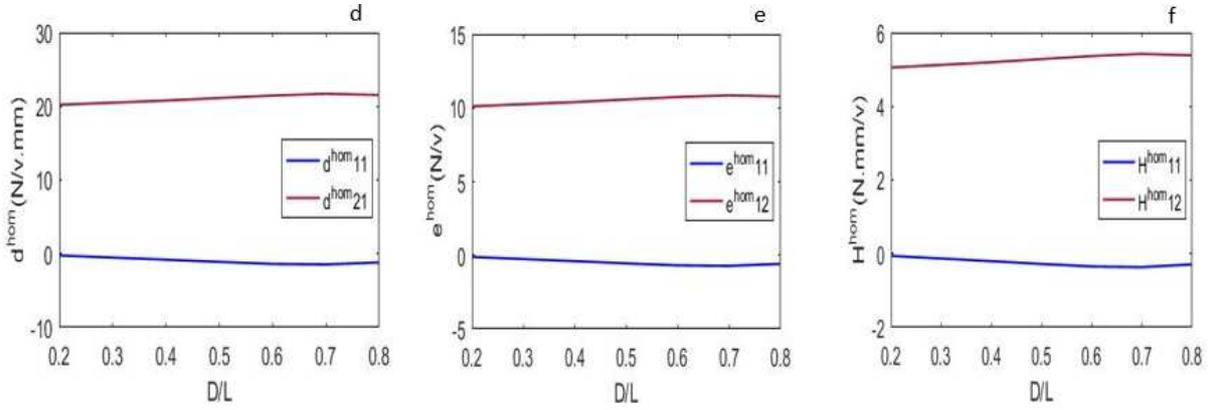
**Fig.9:** Homogenized d) piezoelectric coefficients  $d^{\text{hom}}$ , e) coupling coefficients  $e^{\text{hom}}$ , f) coupling terms  $H^{\text{hom}}$ .
