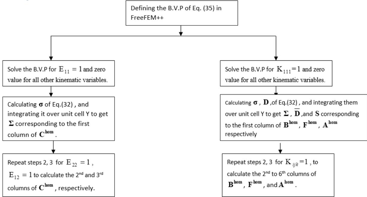
**Fig.2:** Schematic diagram for the computation of the effective moduli  $C^{\text{hom}}$ ,  $B^{\text{hom}}$ ,  $F^{\text{hom}}$ ,  $A^{\text{hom}}$
