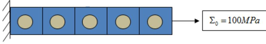
**Fig.4:** 1D flexoelectric beam incorporating many repetitive unit cells along its length
