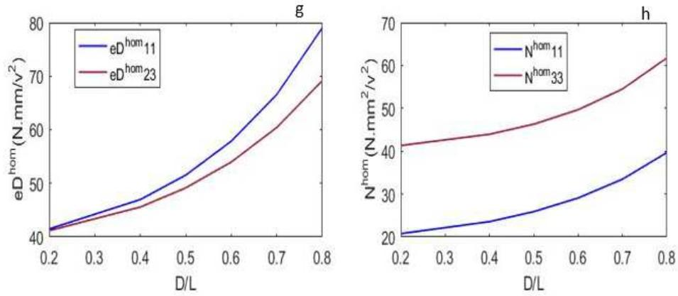
**Fig.10:** Homogenized g) coupling term  $eD^{\text{hom}}$  and h) coupling term  $N^{\text{hom}}$ .
