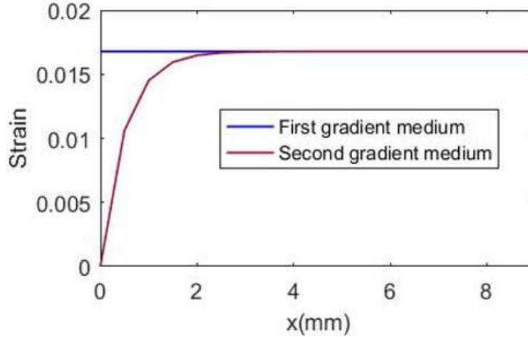
**Fig.6:** Deformation with and without second gradient terms.
