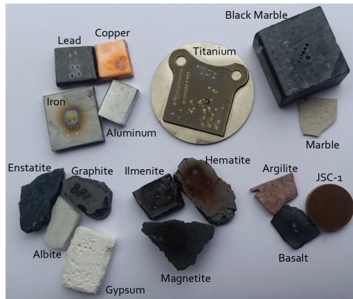
Figure 2: Pictures of all the samples detailed in Table 2. The laser craters created for this study are seen in almost all the targets. For some targets, multiple craters resulting from other experiments can also be seen.
