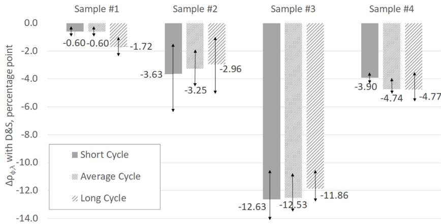
**FIGURE 2.A.** Specular reflectance ( $\Delta\rho_{\lambda,\phi}$ ) losses for samples #1 to #4 in function of their cycle duration
