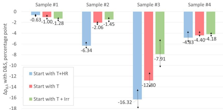
**FIGURE 3.A.** Specular reflectance ( $\Delta\rho_{\lambda,\phi}$ ) losses for samples #1 to #4 in function of the initial stress encountered
