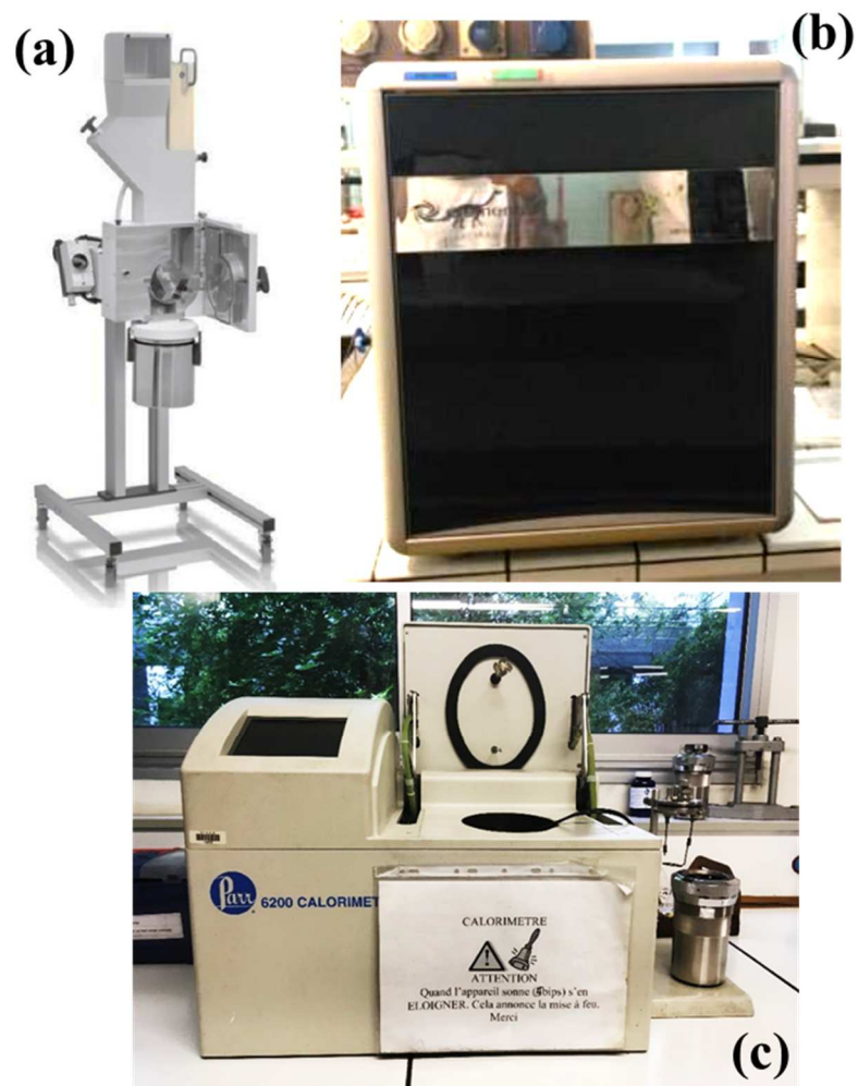
Fig. 3: The various sampling and analysis apparatus used in this study: (a) cutting mill Retsch SM 100, (b) ElementarVario Macro tube CHN analyzer, (c) an Automated Isoperibol Fixed Bomb Parr 6200 bomb calorimeter.
