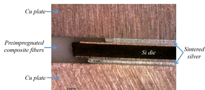
Fig. 1: Cross section view of the PCB Embedded assembly composed by a Silicon 100 V die stacked between two thick copper IMS substrates.
